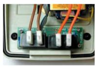
opening under the circuit board and up to the top of the board. The hole can be enlarged as required with a sharp knife. For maximum environmental protection, keep the hole as small as possible and later it can be silicone sealed. Similarly feed the LV mains cables through the rectangular slot, enlarging as required. For maximum safety, ensure LV and ELV cables are segregated.
